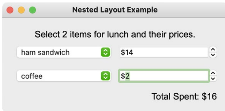
Figure 4-3. Widgets arranged using a combination of layout managers
