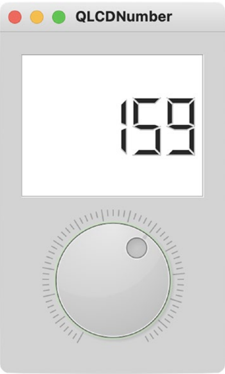
Figure A-1. Example of the QLCDNumber and QDial widgets. The XML and Python code for this example can be found in the Appendix folder of the GitHub repository
