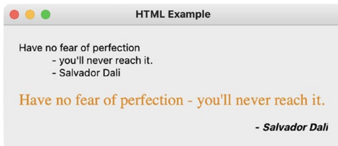
Figure 6-1. Two QLabel widgets display the same text, but the bottom label has been modified
